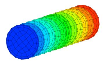
Figure 10.9 Domain for the turbulent pipe flow problem.
