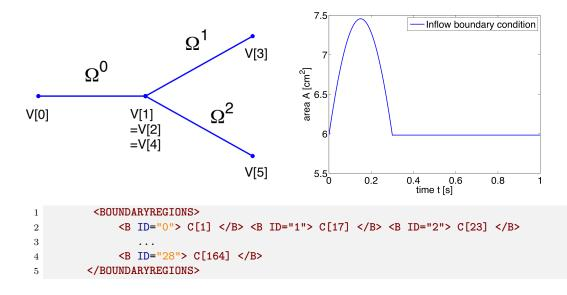
In the boundary conditions section the inflow and outflow conditions are set up. Here we use an inflow boundary condition for the area at the beginning of the ascending aorta taken from [30] and plotted on the right. Potential choices for inflow boundary conditions include Q-Inflow and Time-Dependent inflow. The outflow conditions for the terminal regions of the network could be specified by different models including eTerminal, R, CR, RCR and Time-Dependent outflow.
