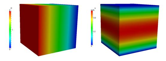
Figure 10.6 Pressure and velocity profiles for the laminar channel flow (full 3D).
