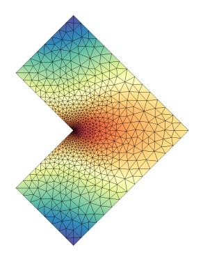
Figure 11.1 Solution of the *u* displacement field for the L-shaped domain.
