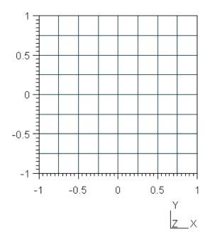
Figure 7.1 Geometry used for the example case of modelling propagation of acoustic waves where  $\bar{u}_i = 0$ ,  $\bar{p} = p_{\infty} = 10^6$ ,  $\bar{\rho} = \rho_0 = 1.204$
