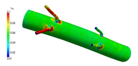
Figure 10.14 Non-dimensional wall shear stress distribution.
