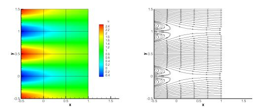
Figure 10.3 Velocity profiles for the Kovasznay Flow (2D).
