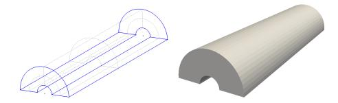
**Figure 4.1** Geometry definition in Gmsh (left) and resulting high-order mesh visualised in ParaView (right).
