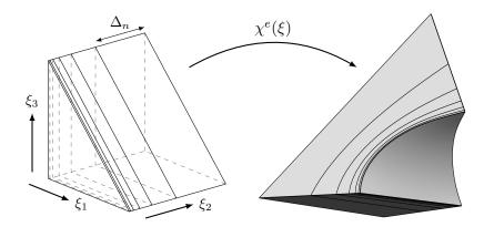
Figure 4.4 Splitting  $\Omega_{st}$  and applying the mapping  $\chi^e$  to obtain a high-order layer of prisms from the macro-element.
