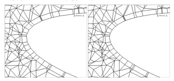
Figure 4.3 (a) Leading edge without spherigons, (b) Leading edge with spherigons
