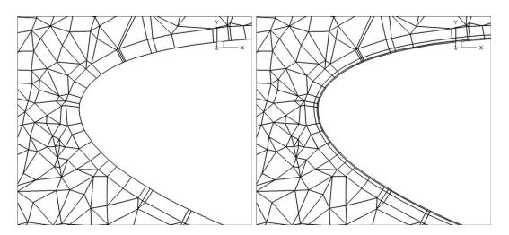
Figure 4.5 (a) LE with Spherigons but only one prism layer for resolving the boundary layer, (b) LE with Spherigons with 3 growing layers of prisms for better resolving the boundary layer.
