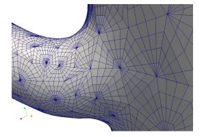
Figure 10.12 Surface mesh indicating curved surface elements at a branch location.
