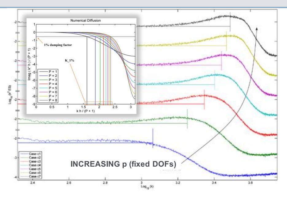
$$\frac{\partial u}{\partial t} + a \frac{\partial u}{\partial x} = \mu \frac{\partial}{\partial x} \left( \mathcal{Q} \star \frac{\partial u}{\partial x} \right) \approx -\mu \sum_{k} k^2 \, \hat{\mathcal{Q}}_k \, \hat{u}_k \, \exp(ikx)$$
