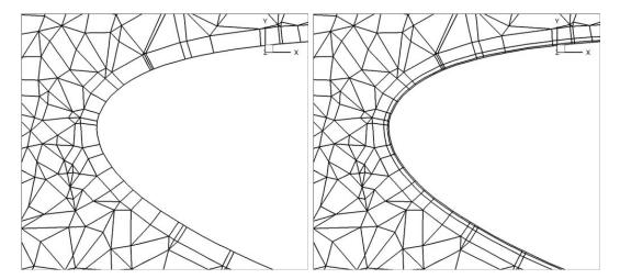
**Figure 10.2** (a) LE with Spherigons but only one prism layer for resolving the boundary layer, (b) LE with Spherigons with 3 growing layers of prisms for better resolving the boundary layer.
