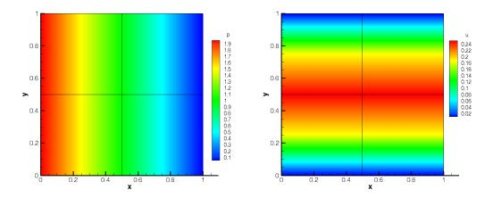
Figure 7.3 Pressure and velocity profiles for the laminar channel flow (2D).
