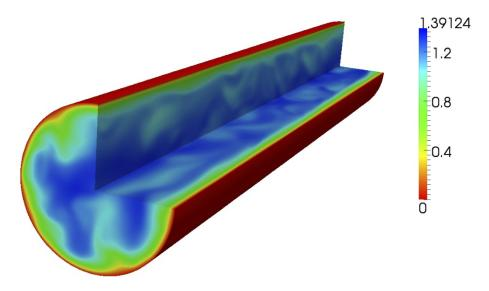
Figure 7.8 Velocity profile of the turbulent pipe flow (quasi-3D).
