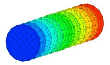
Figure 7.7 Domain for the turbulent pipe flow problem.
