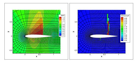
**Figure 6.1** (a) Steady state solution for M=0.8 flow at  $\alpha=1.25^\circ$  past a NACA 0012 profile, (b) Artificial viscosity ( $\epsilon$ ) distribution
