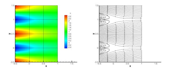
Figure 7.2 Velocity profiles for the Kovasznay Flow (2D).
