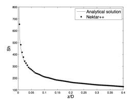
Figure 3.3 Concentration gradient at the surface of the pipe.
