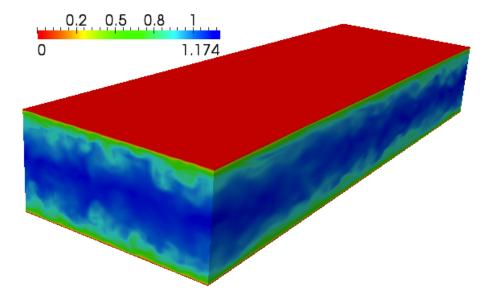
Figure 7.6 Velocity profile of the turbulent channel flow (quasi-3D).
