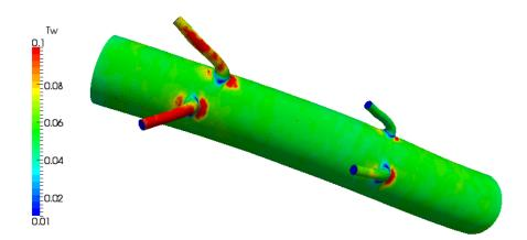
Figure 7.12 Non-dimensional wall shear stress distribution.
