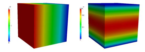
Figure 7.4 Pressure and velocity profiles for the laminar channel flow (full 3D).
