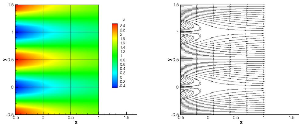
Figure 10.3 Velocity profiles for the Kovaszny Flow (2D).
