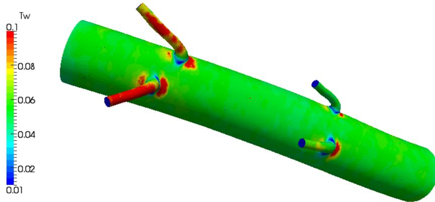
Figure 10.14 Non-dimensional wall shear stress distribution.
