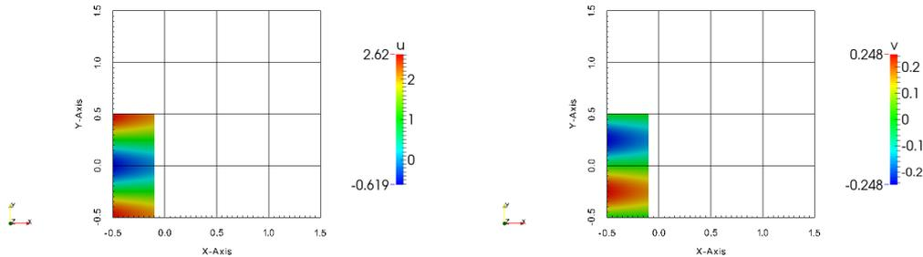
Figure 10.4 Velocity profiles for the Kovasznay Flow in truncated domain (2D).
