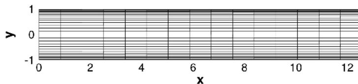
Figure 10.7 Mesh used for the turbulent channel flow.
