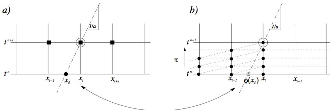
**Figure 10.1** Schematic representation of the substepping approach. (a) Making an explicit time step the hyperbolic solution, travelling with a speed  $a$ , can be understood as being related to the solution at point  $x_d$  (the departure point). (b) Making smaller explicit time steps we can evaluate the solution  $\phi(x_d)$  at the departure point and then use this value to make a semi-Lagrangian discretisation of the implicit components usually associated with diffusion.
