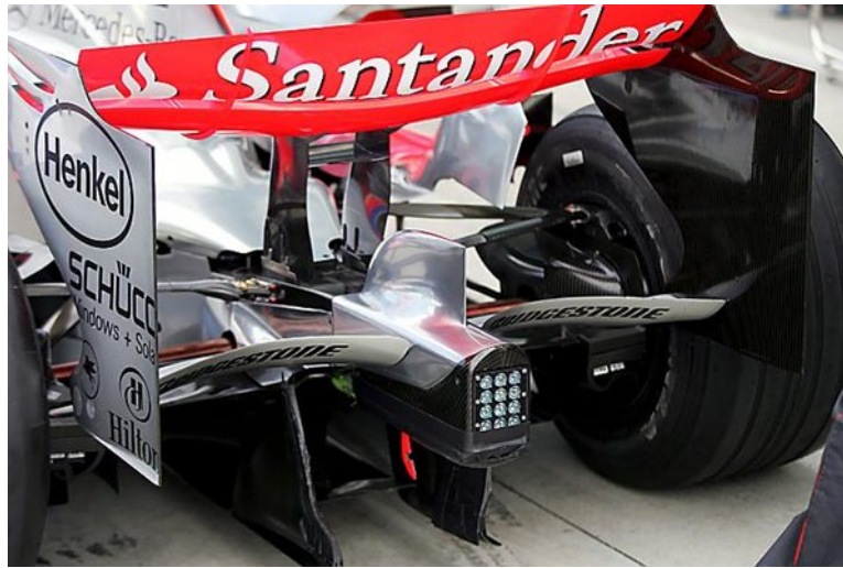
Figure 1.3: Photo of the rear wing trailing edge of McLaren Mercedes MP4/22 (courtesy of McLaren Racing).
